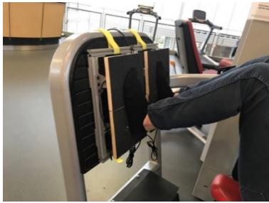
Figure 1. Setup for measuring the force while the participant uses the leg press and attached measuring device.
