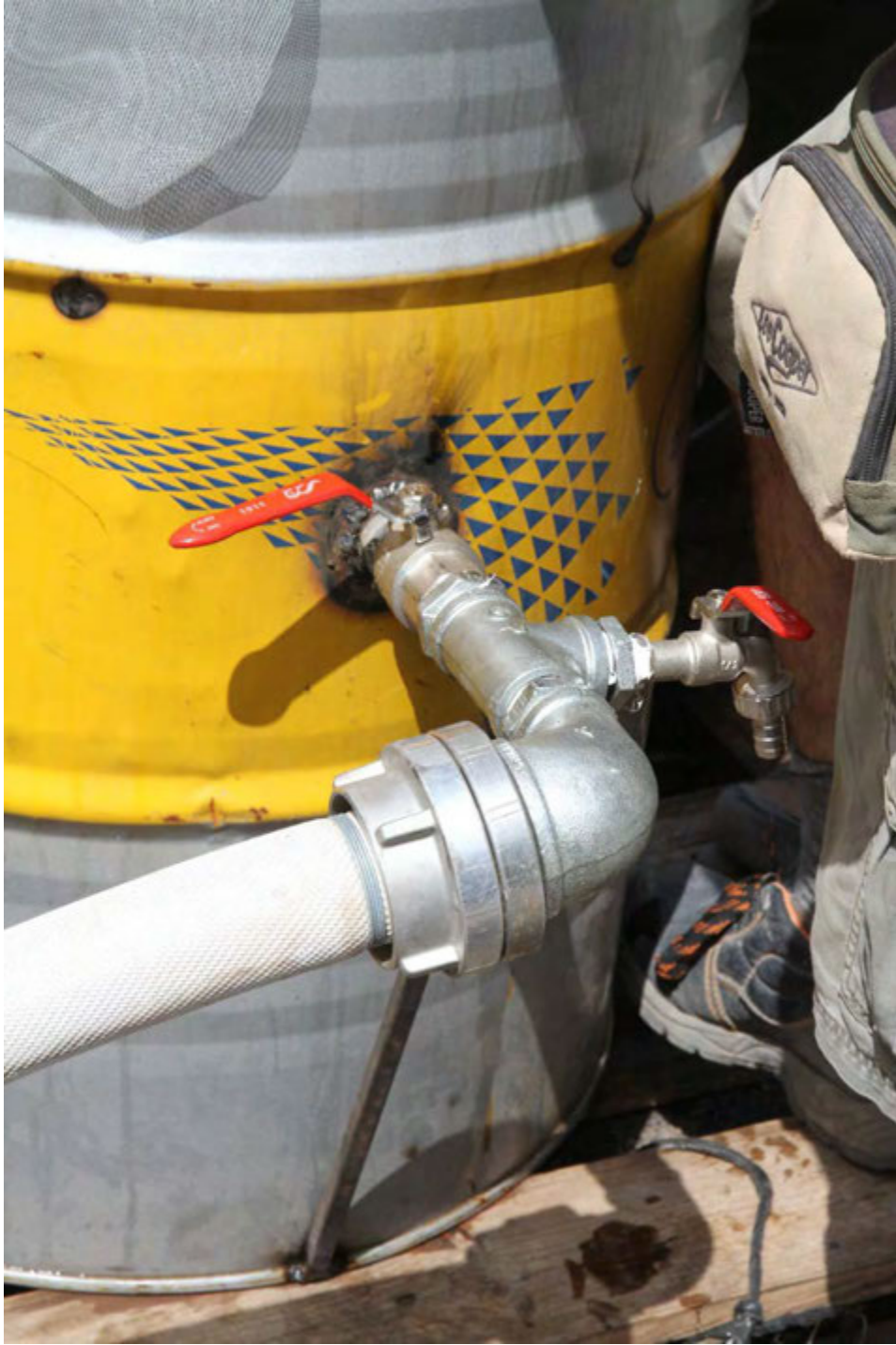
Figure 134, water intake to the device.
