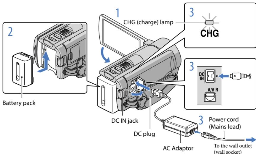
You can charge the “InfoLITHIUM” battery pack (V series) after attaching it to your camcorder.
