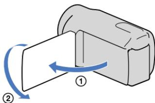
Open the LCD panel 90 degrees to the camcorder (①), then rotate it 180 degrees to the lens side (②).
