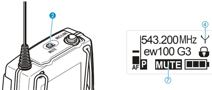
The **MUTE** switch (2) allows you to mute the audio signal or to deactivate the RF signal. Via the "Mute Mode" menu item, you can set the desired function of the **MUTE** switch (2):
