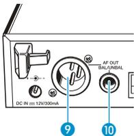
The receiver's XLR-3M socket 9 and the 1/4" (6.3 mm) jack socket 10 are connected in parallel.
