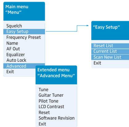
When one of the standard displays is shown on the display panel, you can get into the main menu by pressing the **SET** button **4**. The extended menu “**Advanced Menu**” and the submenu “**Easy Setup**” can be accessed via the corresponding menu items.
