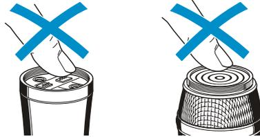
When unscrewing the microphone head during operation, the muting function is automatically activated. "MUTE" appears on the display panel.
