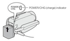
4. When the battery pack is fully charged, disconnect the compact power adapter from the camcorder and then from the power outlet.
