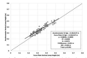
**Figure 1:** Comparison of vertical jump heights determined from the force plate and the experimental accelerometer. Dashed line=line of agreement. Solid bold line=regression line.
