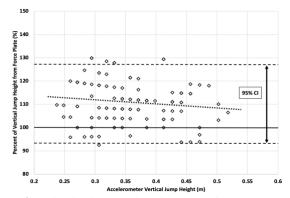
**Figure 2:** Bland-Altman plot demonstrating agreement in vertical jump heights measurements between the force plate and the experimental accelerometer. Dashed lines=95% CI. Dotted line=regression line. Solid bold line=line of agreement.
