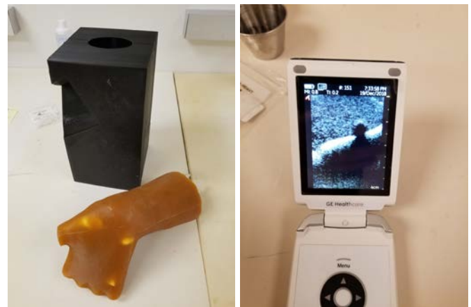
Figure 1: Radial artery simulator model removed from the mold (Left). Scan showing the results of the ultrasound properties when the model is observed (Right).
