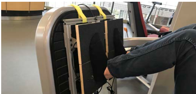
Figure 1: Participant using instrumentation platforms strapped to a standard leg press.
