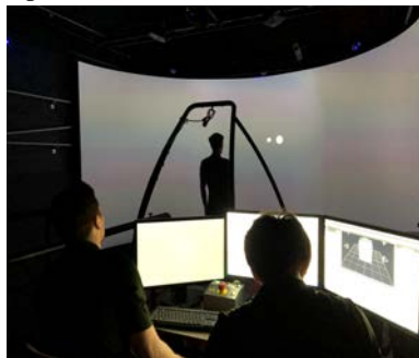
Figure 1: Image of apparatus set-up. Consisting of CAREN and 5-retroreflective markers.
