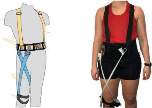
**Figure 1:** Example of a previous design (left) of a unilateral exoskeleton and the design of the proposed exoskeleton (right) [2].
