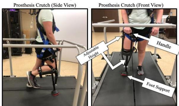
**Figure 1:** The prosthesis crutch intended to simulate walking with a prosthesis
