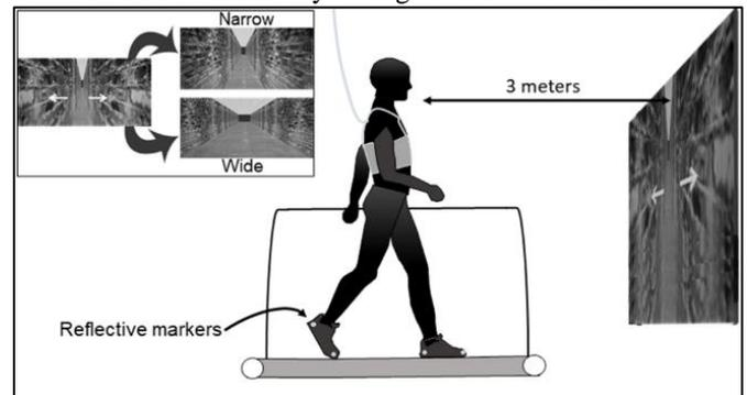
**Figure 1:** Experimental setup showing our width-changing virtual corridor with the Narrow condition (altering between 0.38 m and 1.14 m; left top) and the Wide condition (altering between 0.38 m and 2.67 m; left bottom) identified.
