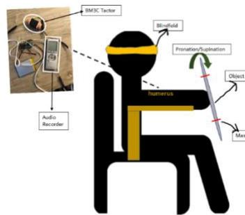
**Figure 2.** Proposed experimental set up. The participant will be blindfolded to ensure proper occlusion of the wielded object. The BM3C tactor will be fastened to the humerus where vibrational stimuli embedded with a noise signal will be applied.
