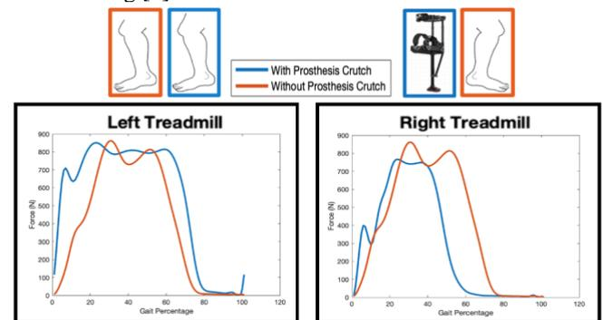
**Figure 2:** The mean of the normalized ground reaction force for walking with (blue) and without (orange) the prosthesis crutch
