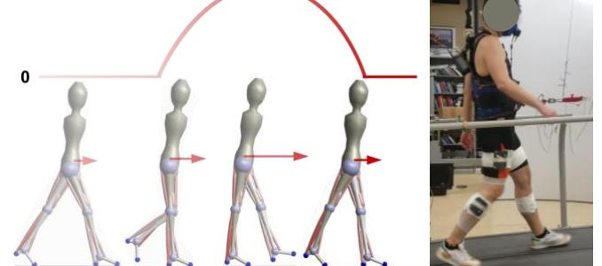
Figure 1: Neuromuscular model and experiment with assistive force at COM
