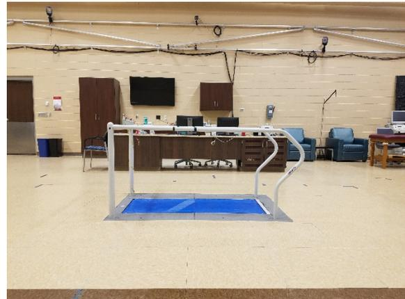
This lab also includes a treadmill that measures foot pressure (KinTread Pressure Treadmill, Noraxon U.S.A. Inc., Scottsdale, AZ, USA) to analyze force and pressure distribution during standing, walking, and running. There is a 10 camera motion capture system with 2 high-speed cameras (OQUS 500/Miqus, Qualisys, Göteborg, Sweden) is housed in this lab as well. This camera system is dedicated to sports biomechanics and includes golf and baseball analysis modules from the manufacturer.
